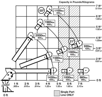
Weight of load handling devices are part of the load lifted and must be deducted from the capacity.
