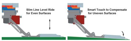
The MBB PALFINGER smart touch flat platform is able to compensate for different loads and terrain while maintaining level during the travel.
