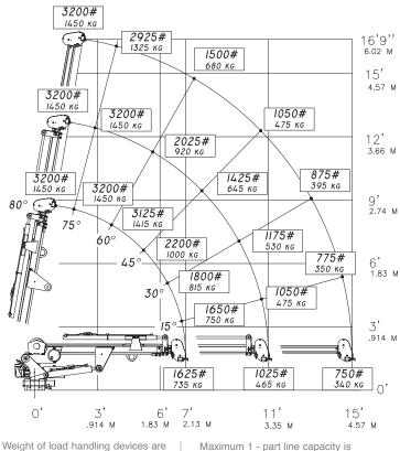
Weight of load handling devices are part of the load lifted and must be deducted from the capacity. Maximum 1 - part line capacity is 1600 lbs. (725 kg). For greater loads, use 2 - part line.
