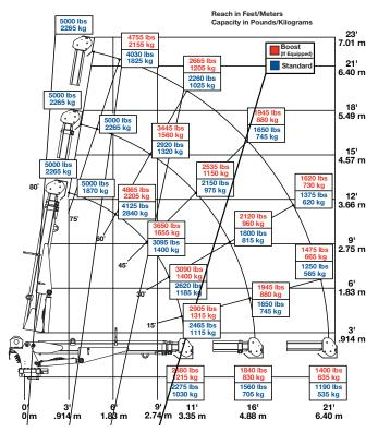
Weight of load handling devices are part of the load lifted and must be deducted from the capacity. Maximum 1-part line capacity is 2500 lbs. (1130 kg). For greater loads, use 2-part line.
