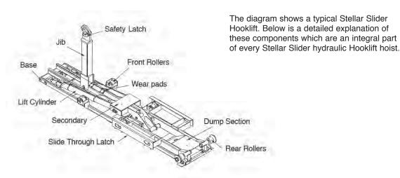
Base Section: The base section of a Stellar Slider may also be called a sub-frame. All Stellar Slider Hooklifts are tied
