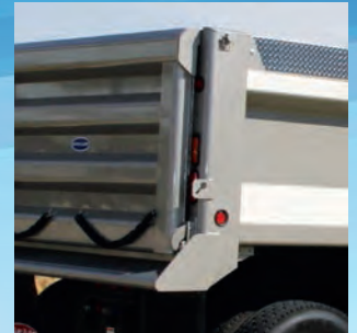
DuraClass bodies come with full depth corner posts and enclosed tailgate hardware.
