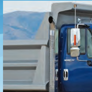
HPT features fully enclosed front corner posts.
