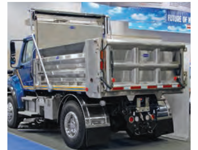
Premium Steel Construction- Minimum 45,000 psi. Additional steel and stainless steel options available.
