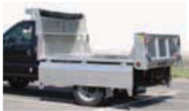
Fold down aluminum sides are lightweight and easy to operate.
