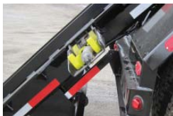
"The Hooker" Securement System at Rear Hinge
