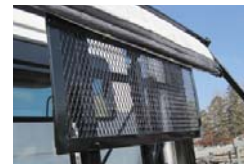
Window Screen Mounted to Tarp System Gantry
