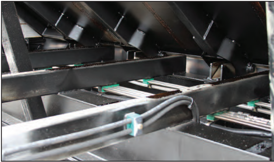
▲ Bolt-On Hinges with Stainless Steel Pins
