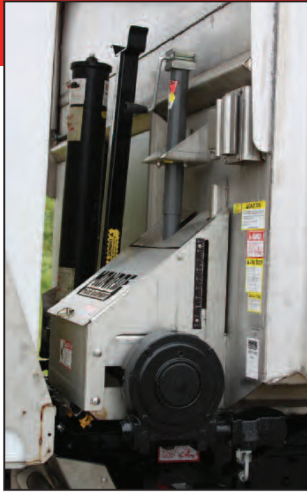
▲ 25:1 Drive System & Screw Adjustable Gate
