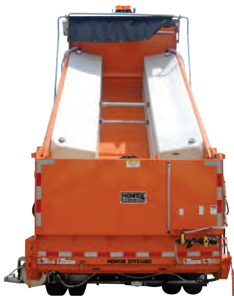
In-Bed Tank Pre-wet System
