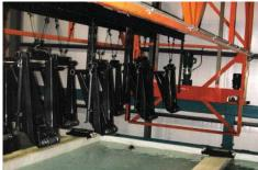
Removed from the bath and rinsed to reclaim undeposited paint solids.
