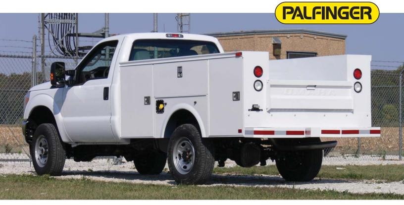
The Omaha Standard PALFINGER 8' service body is designed for a single or dual wheel chassis with 56" CA. Single wheel models have 15" deep compartments and 48-1/2" wide floors as standard. Dual wheel bodies have 20" deep compartments and 54-1/2" wide floors. Standard 96" bodies are 40" high, low-profile models are 36" high, and top opening models are 38" high.
