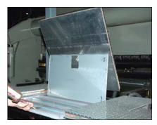
Bonding compartment door panels together with structural automotive epoxy adhesive results in the strongest, most rigid doors of any service body on the market. No welds mean less chance of rusting.
