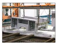
Omaha Standard PALFINGER service bodies receive <u>complete</u> electrocoat prime paint coverage. Because they are e-coated before the doors are installed (unlike the competitors' bodies) Omaha service bodies get total paint coverage, including behind the door hinges. This means superior rust protection in a critical area.
