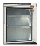
Full perimeter weatherproof automotive bulb type neoprene door seals. Double spring door retainers on full-sized vertical doors to hold doors in positive open or closed position.
