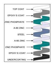
Entire body exterior made from 14-ga A-60 two sided galvannealed zinc coated steel.
