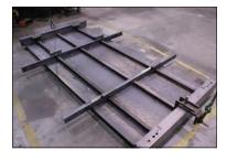
Strongest understructure of any service body - 7ga. full-width formed channel cross members vs. competitor's 11ga. cross members - 50% thicker material. Front cross member reinforced with 7ga. plates at body mounting points. Cross members are bolted to side compartments to give maximum support. Entire body underside has automotive type undercoating.
