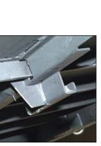
Exclusive vertical "legs" of intermediate cross members rest on truck frame to provide maximum body support in critical wheel well area.
