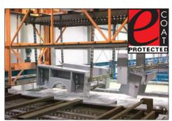
Omaha Standard PALFINGER E-coat completely covers the products to make them durable and corrosion resistant.
