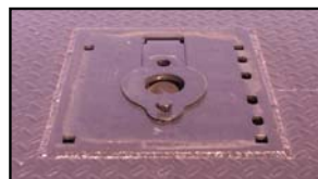
Retractable ball hitch for quick hook ups.
