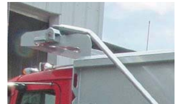
Can be mounted inside cab shield for lower profile. Cab shield then serves as wind deflector
