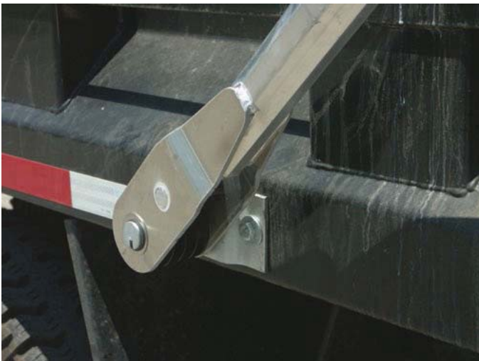
Four spiral spring combination for flipping pressure to accommodate asphalt tarps
