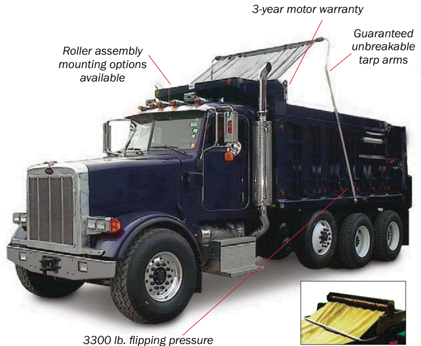
Tarp Saver Bar option locks tarp down on high cab shield mounts
