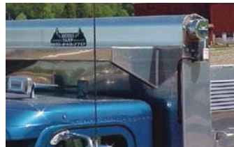
High polish anodized aluminum windshield and end-plates protect the tarp roller; used when not enough room inside cab shield
