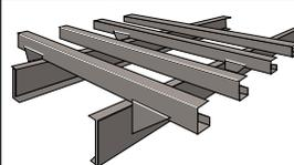
**Rugged Steel Girder Understructure** Two full-length structural steel longitudinal sills reinforced front to rear on both sides by multiple steel gussets. Longitudinal sills and full-width heavy gauge crossmembers are interlocked and welded to the one-piece steel side and end rails.\*\* Understructure is protected by E-Coat primer and a black Powder Coat topcoat
