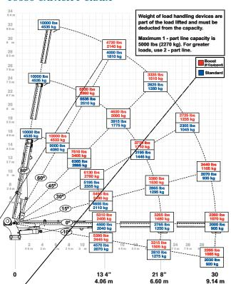
Weight of load handling devices are part of the load lifted and must be deducted from the capacity.
