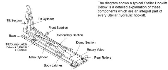
Base Section: The base section of a Stellar Hooklift may also be called a sub-frame. All Stellar Hooklift hoists are tied
