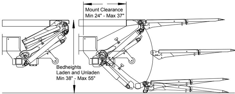
NOTE: 48" and 54" Platform models are available with longer arm for max 55" floor height
