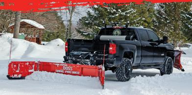
Combine DRAG PRO® 180Z with a front-mounted plow to increase productivity and cut time on the job up to 50%
