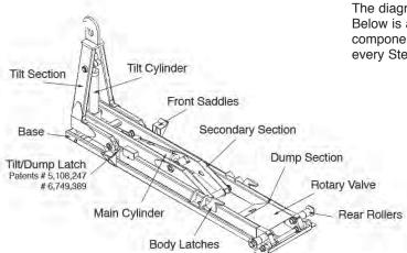
The diagram shows a typical Stellar Hooklift. Below is a detailed explanation of these components which are an integral part of every Stellar hydraulic hooklift.
