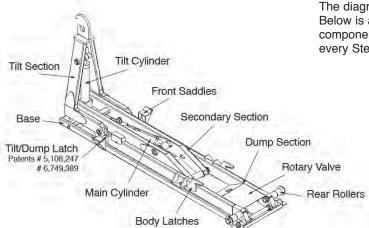
The diagram shows a typical Stellar Hooklift. Below is a detailed explanation of these components which are an integral part of every Stellar hydraulic hooklift.
