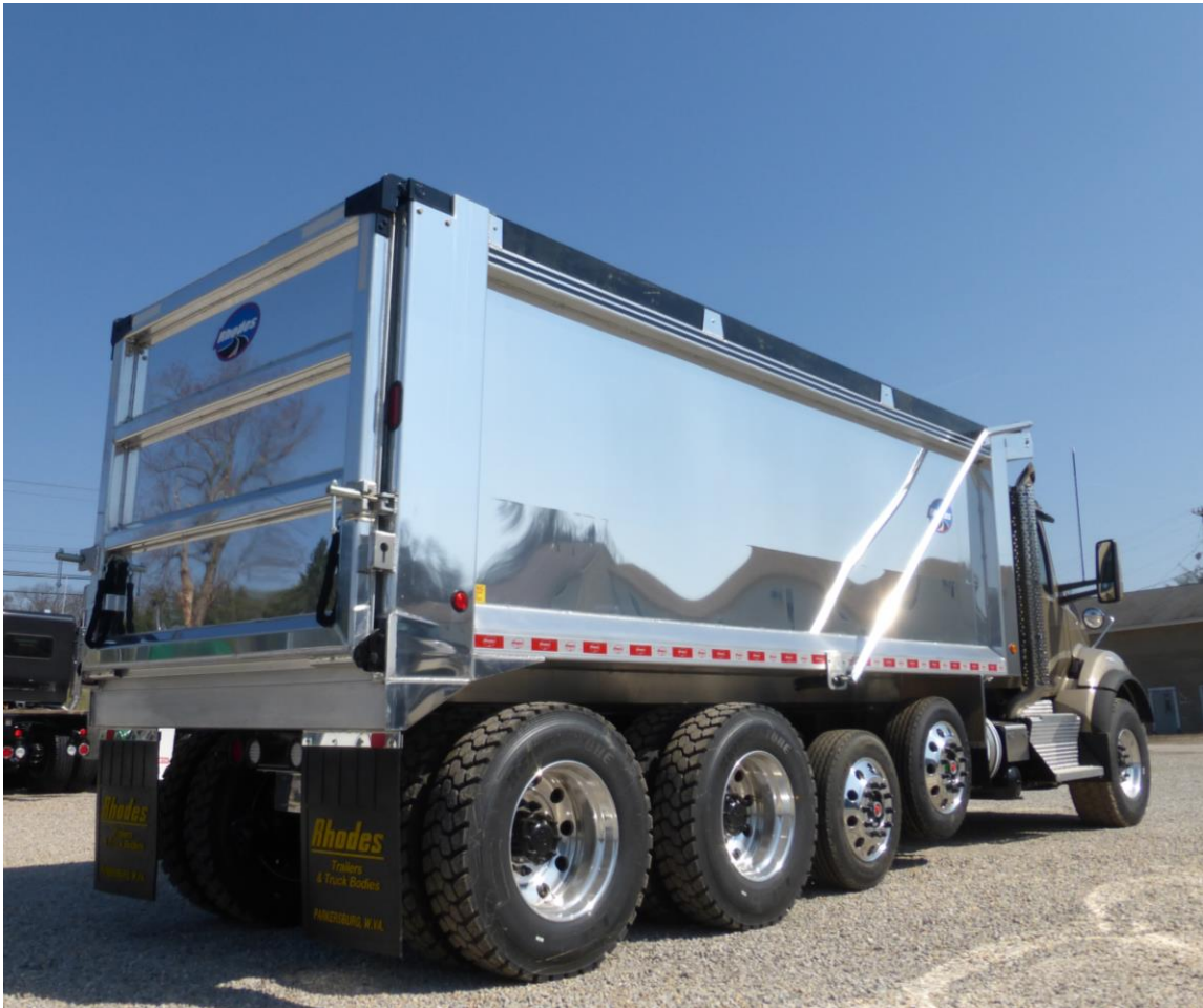
WABF1966-2 ALUMINUM MONOSHELL END DUMP BODY SHOWN
