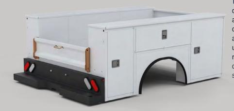
The Service Body (SB) is a traditional weld together design using the same compartment configurations as the CB body. Options include a crane reinforced compartment, transverse front compartment and also a raised front compartment. Side-packs welded to the universal frame/floor eliminates the ability to easily replace the side-packs if damaged. Several bolt on options are available with this option as the overall size of the bodies are the same.
