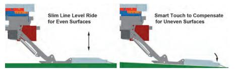
The MBB PALFINGER smart touch flat platform is able to compensate for different loads and terrain while maintaining level during the travel.
