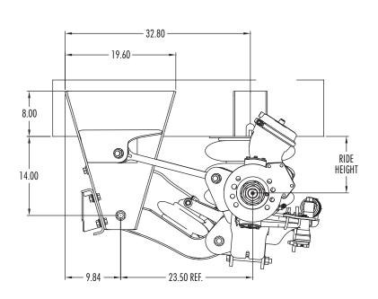
Torque rods angled outward towards rear for better lateral stability
