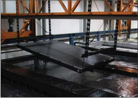
A top coat paint is applied to provide maximum durability and finish.
