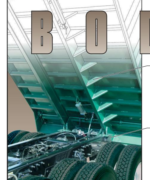
The understructure is manufactured with an 8" channel main frame, 3" channel crossmembers on 12" centers, reinforced with full depth 10 gauge angle braces. Crossmembers are skip welded on each side to the floor, solid welded to the main frame and angle braces. (Optional tubing construction is available)
