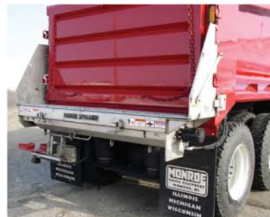
Optional Extended Side Shield Can Eliminate Internal Tailgate Spreader Shields
