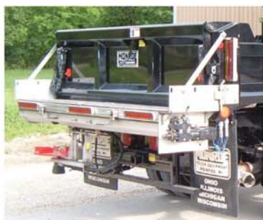
L.E.D Light Bar Assembly for Tailgate Spreader with Stainless Steel Guards S/T/T
