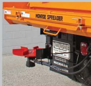
Standard Self Leveling Spinner with Stabilizer Rod
