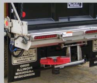
Self Leveling Spinner without Stabilizer Rod
