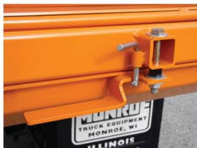
Captive Latching System for Lid and Trough
