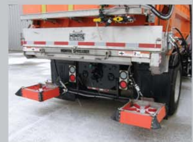
Stationary Bumper Mount Spinners on a One-Way Dual Discharge Spreader
