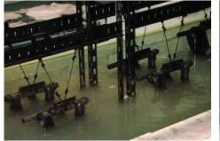
Cleaned and pretreated with a phosphate conversion coating to prepare the product for electrocoating.
