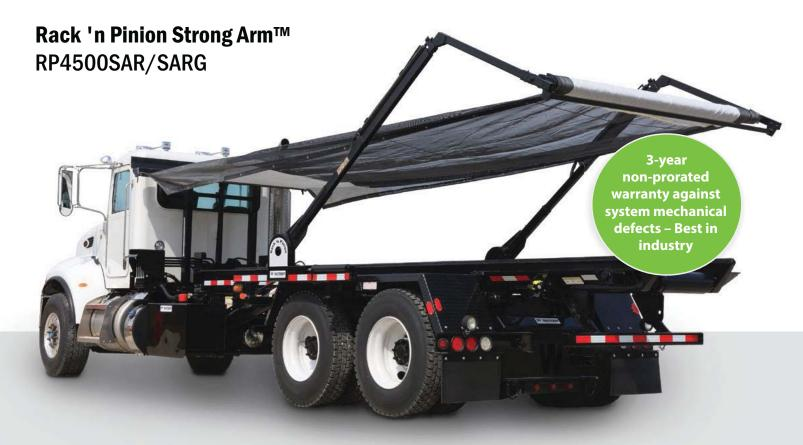
This **Rack 'n Pinion Tarping System** has been the system of choice in the roll-off industry for over ten years. Our patented hydraulic arms and gear assembly combined with our Strong Arm technology and Everlast Tarp Roller produce the only fully hydraulic system known for reliability and low maintenance. The Strong Arm concept uses a greatly strengthened base arm which attaches to the Rack 'n Pinion pivot. The extended "C" Channel provides better leverage, greater control and longer life.
